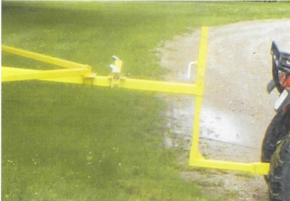
Long Braces – from the flat plate to the brace holder on the wings
